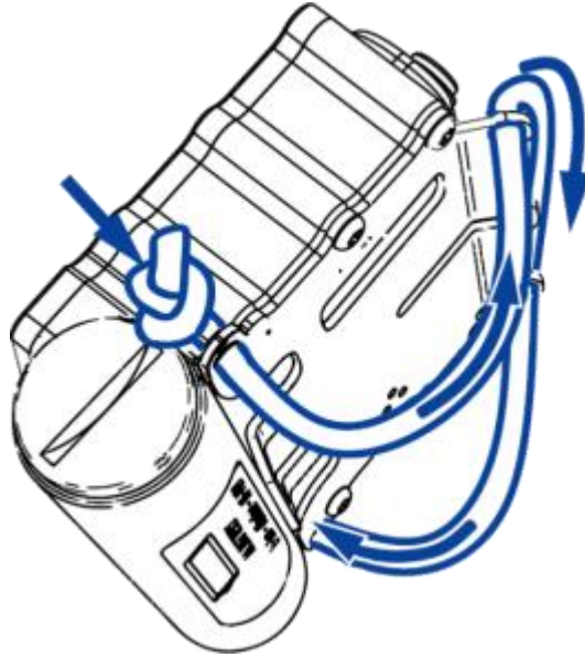
Fig 2 - Bungee cord install
